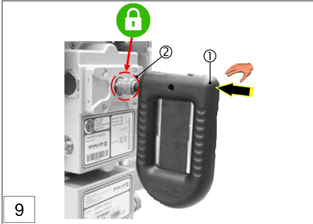
Fig.: 84 : Replacing the VN2020 measuring head (steps 1-9)
