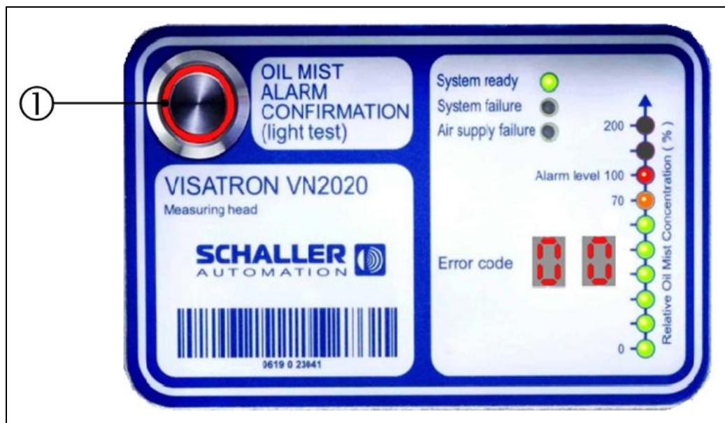
Fig.: 73 : VN2020 measuring head: Confirming an oil mist alarm
