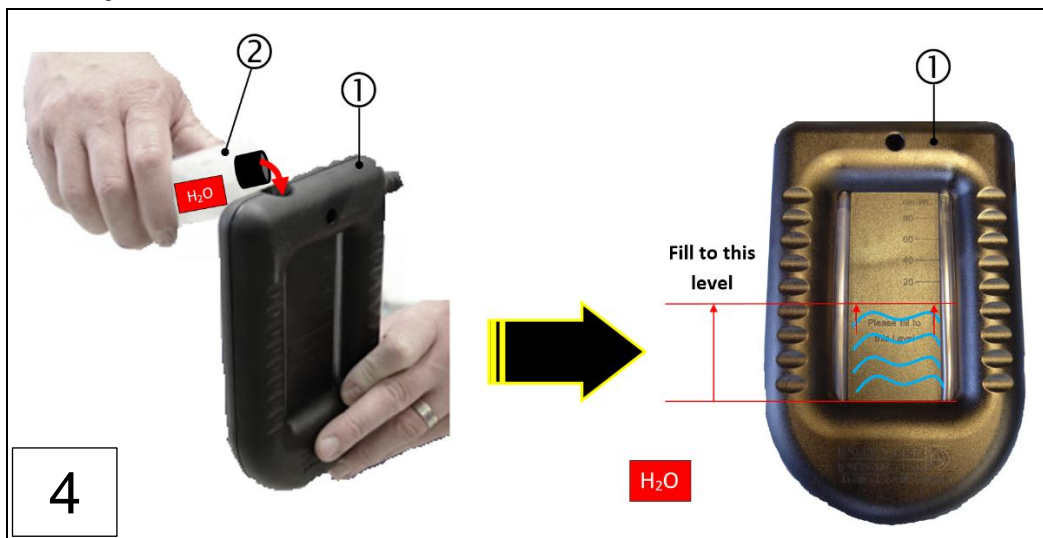
1: U- Rohr- Manometer
