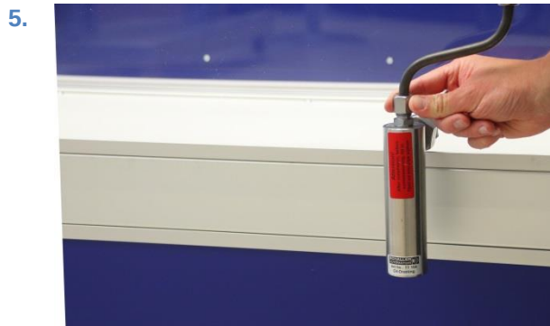
Figure 40: Connection of pipe
