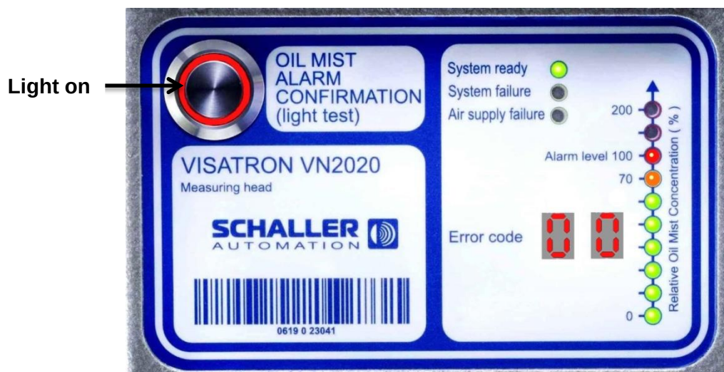
Figure 61: Display with detected oil mist
