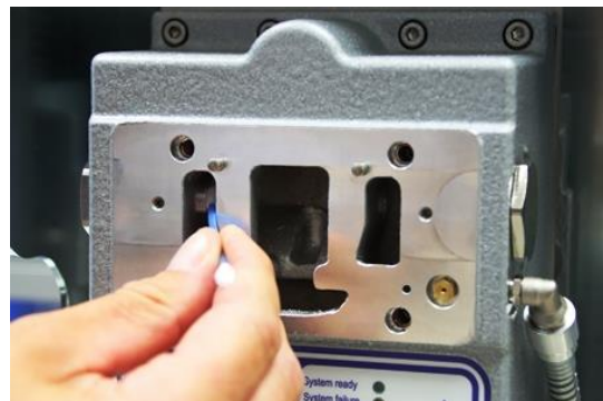
Figure 67: cleaning transmitter diode
