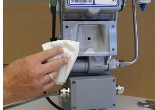
Figure 86: clean sealing surface
