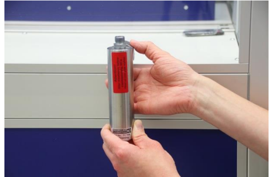
Figure 37: Mounting of pipe siphon
