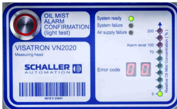
Figure 60: Measuring head display – normal operating mode
