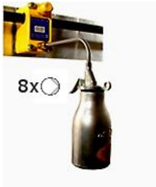
Figure 33: Pumping of lubrication oil
