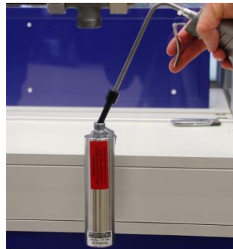
Figure 39: Filling the pipe siphon
