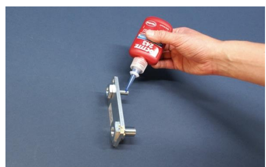
Figure 24: Screws with Loctite
