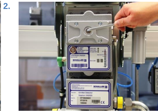
Figure 181: Inspection cover with mounted quick coupling cover
