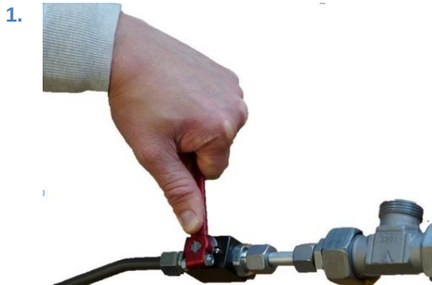
Figure 154: switch off compressed air
