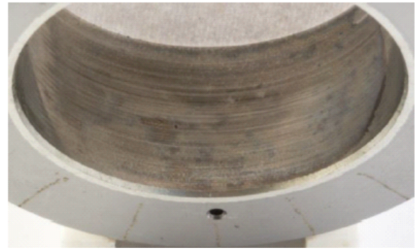
Example of a worn-out plain bearing
